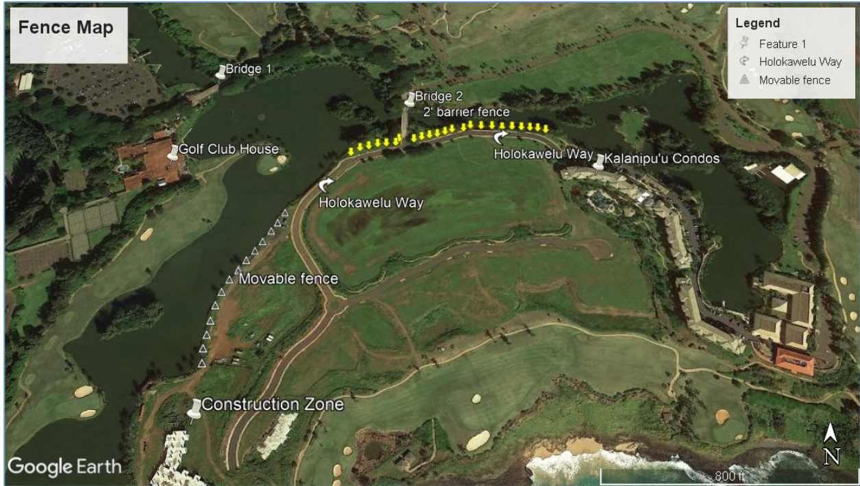
Figure 16 – Bridge 2 Intersections With Holokawelu Road, as well as the semi permanent gallinule fence and the portable fencing. Yellow down pointed arrows represent the location of the semi-permanent fencing, and the hollow white triangle represent the movable section of bird fencing
