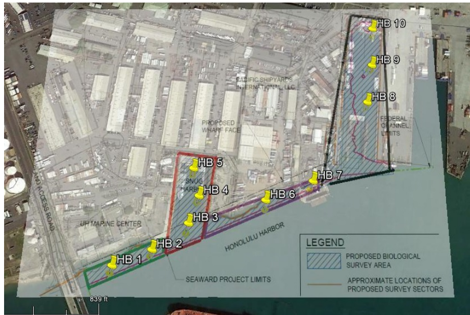
Figure 6. Location of randomly selected deep water harbor bottom survey locations (HB1-HB10) with overlay of project area and dredging limits.
