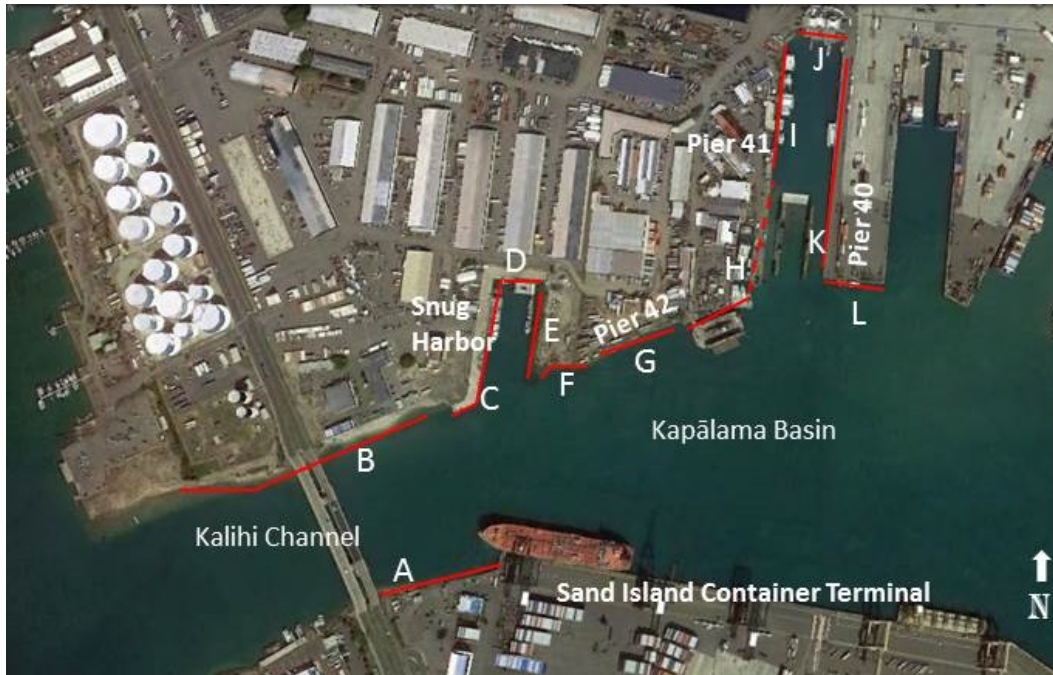
Figure 3. Survey sectors lettered A through L marked with red lines. Dashed line at Sector H indicates part of Sector H not surveyed due to work on the dry docks.
