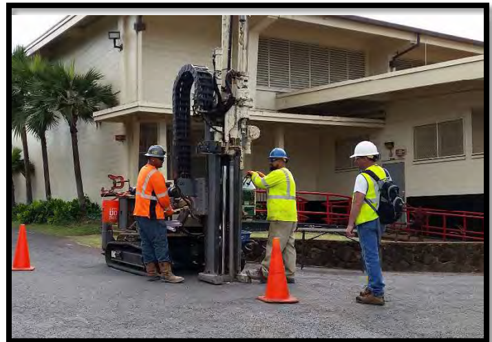
Photograph 1: Sample collection using direct push drill rig at Radford High School
