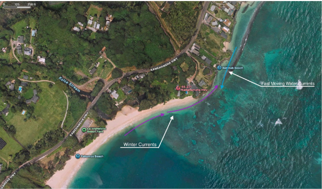
Figure 3-7: Currents Allowing Sand Accumulation at "Bathtub Beach"
