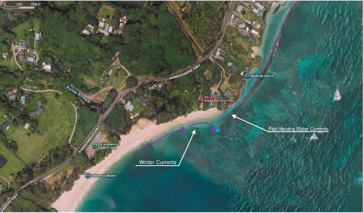
Figure 3-8: Competing Currents not Allow Sand Pass Point
